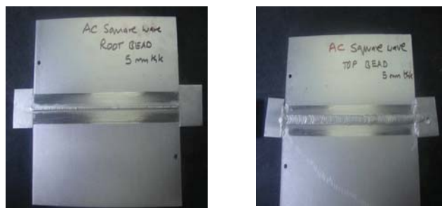
Fig.6 Welded joints by ac Square wave welding
